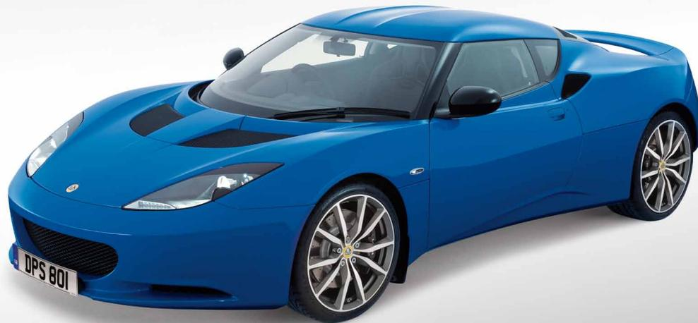
The Evora S blends the sublime handling attributes of the Lotus Evora with the surging linear power of a supercharged V6 engine. Delivering even more attitude, the forced induction power plant delivers 345 hp and 295 lbft of torque. There's no appreciable weight gain: at 1,437 kg the Evora S is still lightweight, muscling from 0 to 60 mph in 4.4 seconds, powering to its 178 mph maximum.
