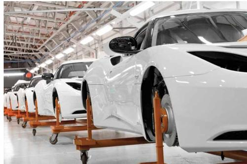
The state-of-the-art Evora chassis is composed of an extruded and bonded aluminium structure, developed for its lightweight yet incredibly stiff design, with a central tub containing the driver's cockpit and safety cell - a format closely reflecting the layout and construction of modern-day racing cars. Its unique design ensures a chassis so stiff that it takes 27,000 Nm to twist it just one degree.
