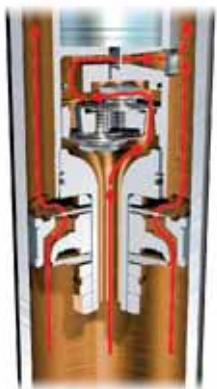
Compression in Normal mode— damper piston with bypass valve open
