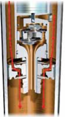
Rebound in Sport mode— damper piston with bypass valve closed
