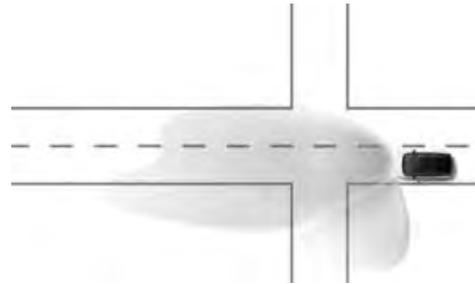
**Cornering Lights<sup>1</sup>.** Light up the dark areas headlight beams don't cover on corners (up to 40km/h).
