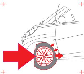
**The wheel as a deformation element:** in a head-on collision, the front wheels are supported by the side member, which absorbs a substantial portion of the impact energy.
