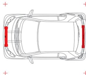
**Crash boxes:** steel deformation elements at the front and rear of the smart fortwo absorb energy from minor collisions at low speeds, ensuring that the tridion safety cell remains undamaged. Furthermore, a damaged crash box is simple to replace.
