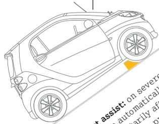
**Hill start assist:** on severe slopes, this feature automatically locks the wheels momentarily after the brake pedal is released, preventing the car from rolling backwards.
