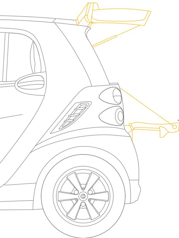
**Twin-section tailgate:** by pressing the unlock button on the 4-button key, the rear window of the coupe can be unlocked from afar and heavy items can be loaded through the top window, even in tight parking spaces, without opening the tailgate.
