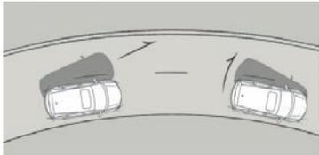
**STABILITY AND CONTROL** THE BEST COLLISION IS THE ONE THAT DOESN'T HAPPEN. IT'S WHY ACURA HAS DEVELOPED AN ARRAY OF SAFETY FEATURES DESIGNED TO HELP YOU STAY OUT OF HARM'S WAY. THESE INCLUDE VEHICLE STABILITY ASSIST™ (VSA®), WHICH CAN DETECT UNDERSTEER OR OVERSTEER AND HELP KEEP YOU ON YOUR DESIRED PATH, ABS BRAKES WITH BRAKE ASSIST THAT CAN SENSE EMERGENCY BRAKING AND DELIVER MAXIMUM BRAKE FORCE, AND A TIRE PRESSURE MONITORING SYSTEM<sup>6</sup> (TPMS).
