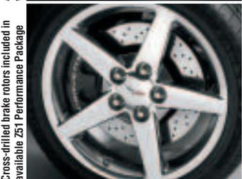
Cross-drilled brake rotors included in available Z51 Performance Package
