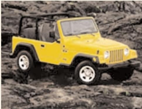
The Wrangler X, with standard 190-horsepower 4.0L Power Tech I-6 engine, five-speed manual transmission and AM/FM stereo radio with cassette player, can really take you places.
