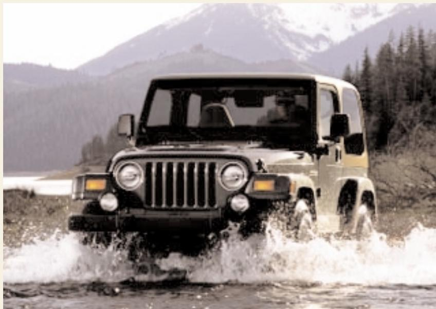
All Jeep<sup>®</sup> prototypes must pass the rigors of Jeep durability testing — off-road and on. One of the extreme off-road test cycles includes repeatedly fording more than 20 inches of water. Wrangler Sahara shown in Shale Green.
