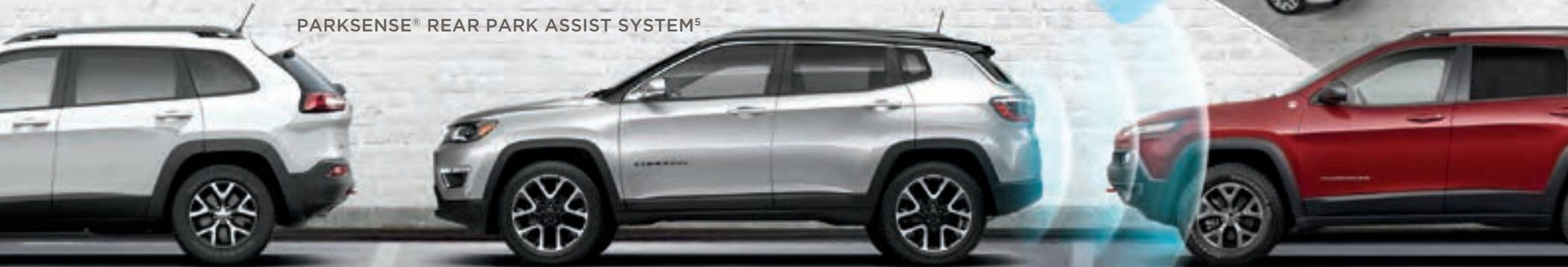
**PARKSENSE<sup>®</sup> REAR PARK ASSIST SYSTEM<sup>5</sup>** This system uses rear ultrasonic sensors to determine relative distance to objects in your back-up pathway. Read-outs in the Driver Information Display notify the driver of rear-object proximity. Available.
