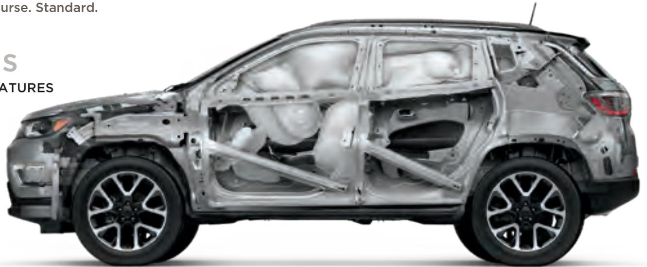
**A Secure Air Bag<sup>8</sup> System** Your need for security is fully respected with this all-around air bag<sup>8</sup> system. Full-length side-curtain, seat-mounted side thorax, and advanced multistage front and driver's inflatable knee bolster air bags<sup>8</sup> all work together to help provide protection. Standard.
