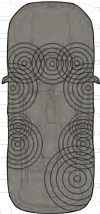
The Premium Alpine® Speaker System is known for its outstanding tonal balance and definition. This system helps create a haven of audio enjoyment, delivering an impressive, realistic sound experience. It features a 12-channel, 506-watt amplifier and nine perfectly placed speakers (including a dual voice coil, 8-inch subwoofer) that work together in perfect harmony. Available.
