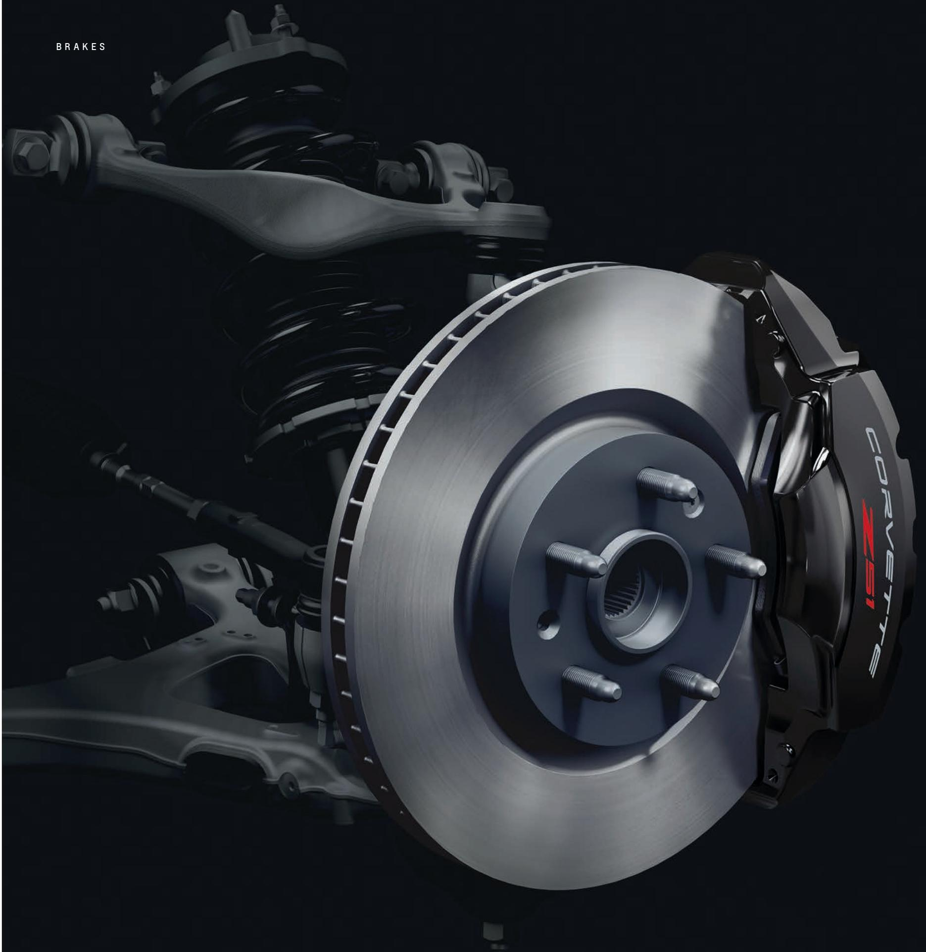
For the first time ever, Stingray uses an electro-hydraulic boost braking system. It adopts the proper pedal feel for each selected driving mode. It also helps reduce pad wear and brake pulsation.
