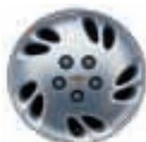
15" x 6" steel wheel with composite bolt-on full wheel cover. Standard on Value, Plus and LS models.
