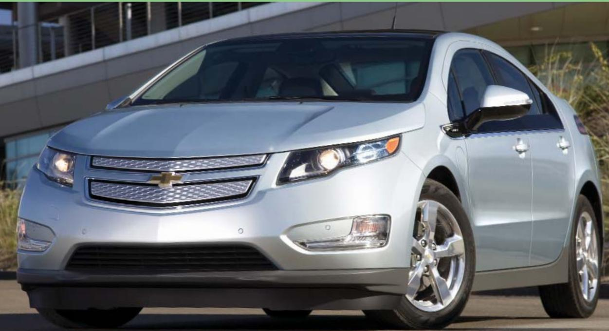
The Chevrolet Volt is an electric vehicle with extended-range capability. It is designed to drive up to 40 miles (assumes fully charged battery) on electricity without using gasoline or producing tailpipe emissions. When the Volt's lithium-ion battery is depleted, an engine/generator seamlessly operates to extend the total driving range to about 300 miles. Production begins late this year.
