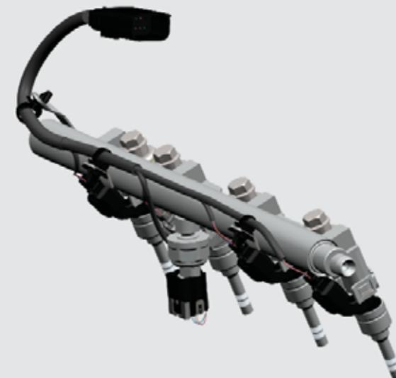
With direct injection, the fuel is injected directly into the cylinders. Vaporization of the fuel within the cylinder lowers the temperature of the air and fuel mixture which reduces engine knock. Less knock allows increased compression ratio, which in turn increases peak engine power and improves overall fuel efficiency.
