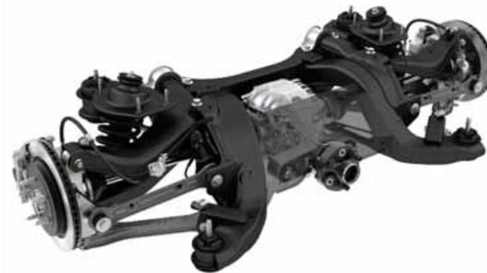
Standard on V8 models and on V6 manual models, a limited-slip differential helps to improve traction by directing engine power to the rear wheel with the best traction. This gets the power to the ground for enhanced performance, especially in low-speed corners and low-traction conditions.
