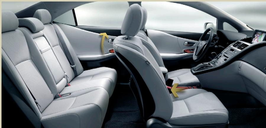
In certain rear-end collisions, active front headrests<sup>24</sup> raise upward and forward, helping to reduce the severity of a whiplash injury.
