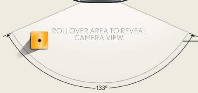
Using a specially designed wide-angle lens to help reveal hard-to-see areas, an available Wide-view Front Monitor<sup>5</sup> comes on at the touch of a button (or automatically, if you choose) when you're driving at low speeds. A camera mounted in the grille displays a 190-degree front view on the navigation screen.
