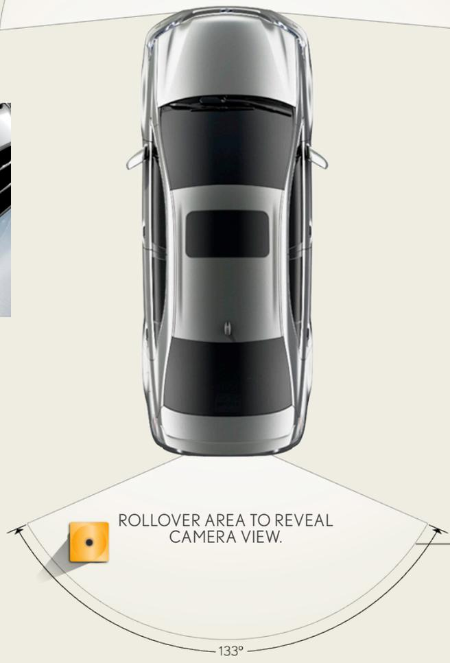
Using a specially designed wide-angle lens to help reveal hard-to-see areas, an available Wide-view Front Monitor<sup>5</sup> comes on at the touch of a button (or automatically, if you choose) when you're driving at low speeds. A camera mounted in the grille displays a 190-degree front view on the navigation screen.
