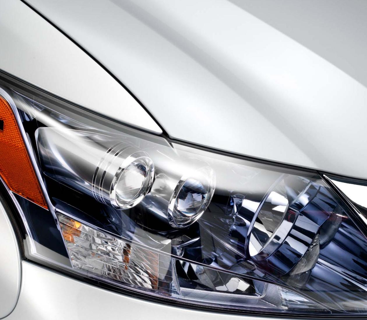
The best way to improve vision is to outthink what impairs it. Enter the available LED Dual-swivel headlamps with Adaptive Front Lighting System (AFS). It enables the LED headlamps to turn so they're better able to illuminate curves. They're even capable of independent thought. At speeds above 19 mph, both headlamps swivel into a curve, illuminating more of the road ahead. At lower speeds, the left headlamp rotates up to 15 degrees while the right headlamp rotates up to 10 degrees.
