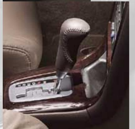
A 4-speed electronically controlled automatic transmission is standard in all Outback H6-3.0 models. The gated shifter provides precise control for manual gear shifting, if desired.
