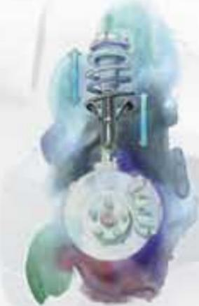
As the body of a vehicle leans in a turn, the suspension of the inside wheel lengthens. All Outback models except Outback Sport feature a rebound spring inside the front strut that is designed to use the mass of the wheels, tires and brakes to resist this lengthening, reducing body roll in turns. The rebound spring also works to reduce the lift of the nose of the vehicle on acceleration.
