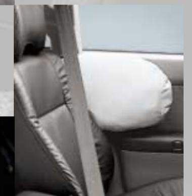
Standard on Outback Limited and Outback H6-3.0 models,\* front seat side-impact air bags are mounted on the front seats, maintaining optimal placement regardless of seating position.\*\*
