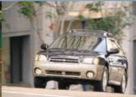
When going uphill, the vehicle's weight shifts rearward, reducing traction to the front wheels. In response, Subaru AWD can smoothly direct power to the rear wheels where there is more traction.
