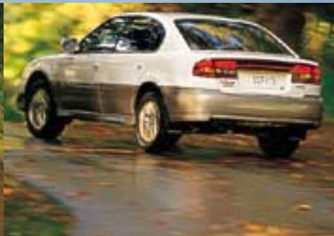
Coming out of a corner, a front-wheel drive car tends to understeer, or plow toward the outside of a curve when accelerating. With AWD, a Subaru vehicle exits a curve with the right amount of power to the rear wheels.
