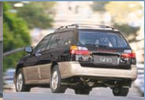
When going downhill, the vehicle's weight shifts forward, reducing rear-wheel traction. Subaru AWD can respond by sending power to the front wheels for better overall steering control and braking performance.
