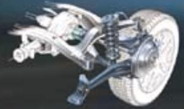
The Outback Sport features a rugged dual-link suspension. All other Outback models feature a rear multi-link suspension designed for exceptional stability – and to help keep handling consistent whether the vehicle is heavily loaded or not. Front and rear stabilizer bars help keep body roll in check.
