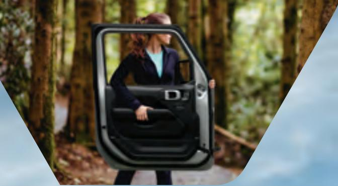
**REMOVABLE<sup>2</sup> DOORS** Just a few easy steps and you're enjoying a full-on open-air experience. These removable<sup>2</sup> doors are made of lightweight aluminum and designed to facilitate easy removal.<sup>2</sup> They feature exposed door hinges with a T50 imprint calling out the Torx<sup>®</sup> bit (included) needed to remove<sup>2</sup> door bolts, a quick-disconnect check strap, and detects to hold the door open.
