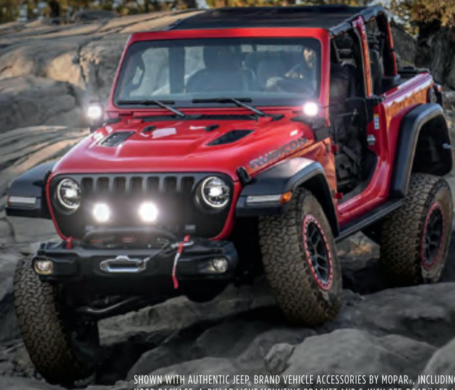
SHOWN WITH AUTHENTIC JEEP, BRAND VEHICLE ACCESSORIES BY MOPAR®, INCLUDING MESH SUN BONNET, RUBICON® HOOD PACKAGE, A-PILLAR LIGHT MOUNTING BRACKET AND 5-INCH OFF-ROAD<sup>27</sup> LED LIGHT KIT, WINCH GUARD LIGHT MOUNTING BRACKETS AND 7-INCH OFF-ROAD<sup>27</sup> LED LIGHT KIT, SATIN BLACK GRILLE, WINCH GUARD HOOP, RUBICON STEEL STUBBY BUMPER, 2-INCH LIFT KIT WITH FOX® SHOCKS, RUBICON FENDER FLARES, JEEP PERFORMANCE PARTS ROCK RAILS, 17-INCH BEADLOCK WHEELS AND BLACK FUEL-FILLER DOOR.
