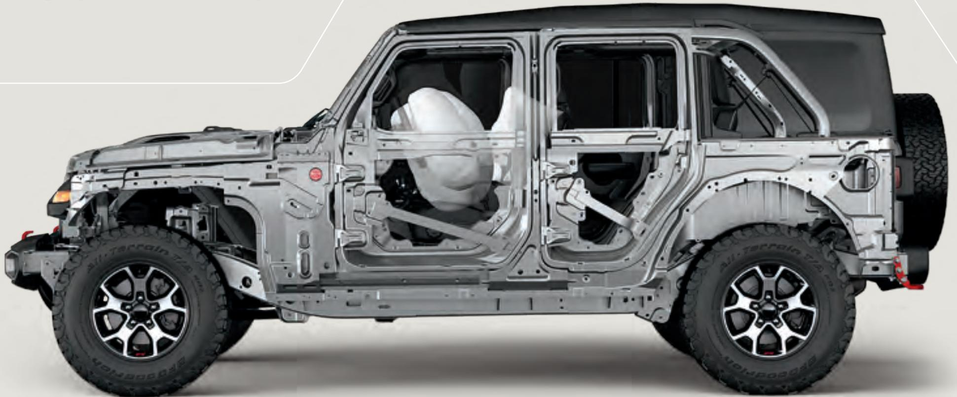
**BODY STRENGTH** The exceptionally solid safety cage consists of high-strength steel paired with lightweight aluminum, making Wrangler lighter in weight while still providing a very strong chassis. Standard.
