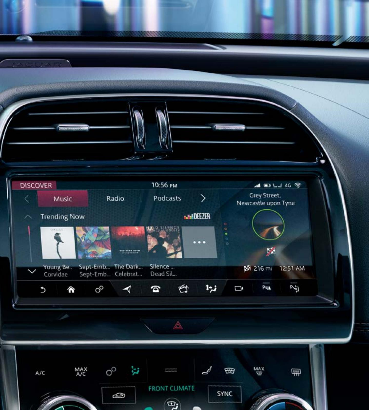
Touch Pro Duo<sup>1</sup> is our innovative twin-screen system, part of Jaguar InControl® technologies, providing a 10" upper Touchscreen and 5.5" lower Touchscreen. The benefit of having a lower screen is to allow dual-tasking, for example, navigation mapping on the upper screen and climate controls and access to other features – such as entertainment – on the lower screen\*.
