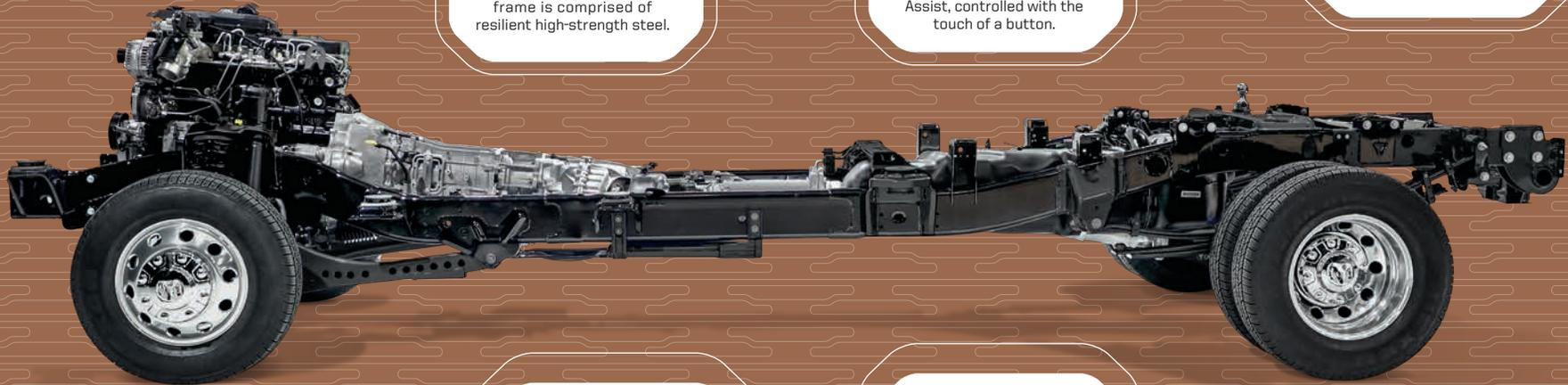
On 4x4 pickup models, a 9.25-inch front axle features new pinion seals; a new axle housing helps reduce Noise, Vibration and Harshness (NVH).
