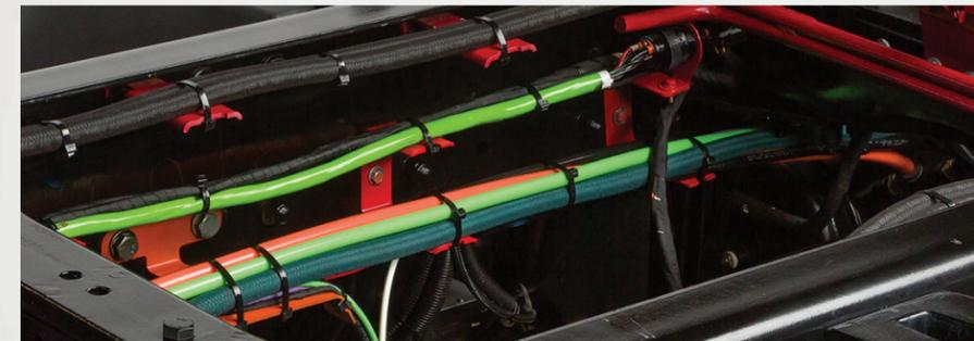
*Fuel, air and electrical lines run the length of the truck and are individually grouped and organized to facilitate quick identification for maintenance.*
