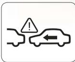
City Safety\* functions at speeds up to 30 mph. This system can help prevent a collision if the difference in speed between your vehicle and the vehicle ahead is less than 9 mph.
