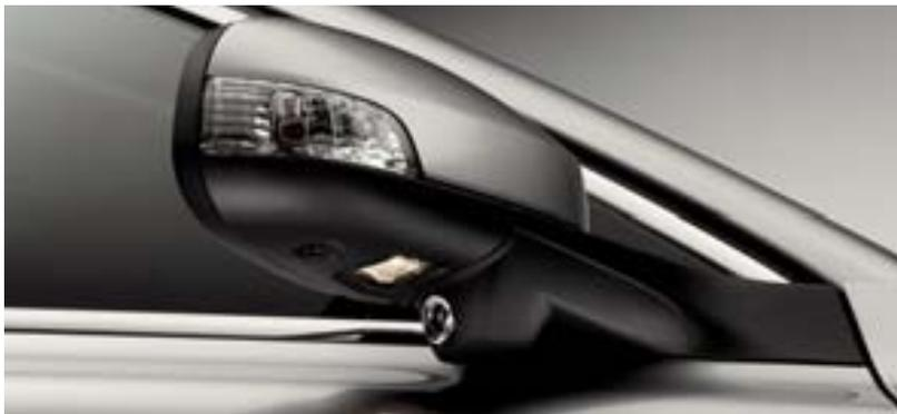
**Power retractable door mirrors with ground lighting**
