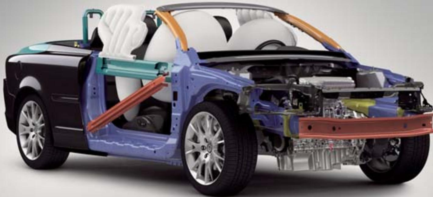
**IN A REAR IMPACT** the rear deformation zones will help absorb crash energy. The fuel tank is designed to remain well protected in front of the rear axle. The head restraints help protect the neck and spine, and Volvo's unique Whiplash Protection System (WHIPS) cradles the front seat occupants in a controlled manner to help prevent whiplash injuries.
