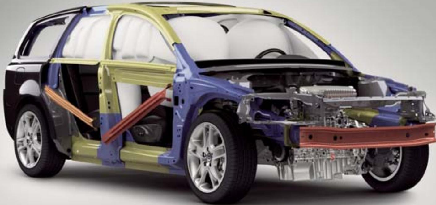
**In a rear impact** the rear deformation zones will help absorb crash energy. The fuel tank is designed to remain well protected in front of the rear axle. The head restraints help protect the neck and spine, and Volvo's unique Whiplash Protection System (WHIPS) cradles the front seat occupants in a controlled manner to help prevent whiplash injuries.
