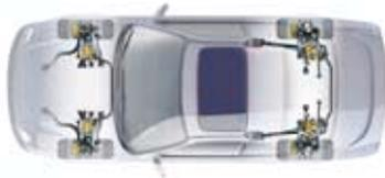
Prelude's race-bred **4-wheel double wishbone suspension** positions the wheels and tires for optimum control and excellent handling, yet also provides a very smooth and comfortable ride.
