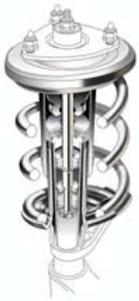
Honda Progressive Valve (HPV) shock absorbers automatically adjust to road and driving conditions, providing softer damping over bumps, firm control when cornering and better stability at highway driving speeds.
