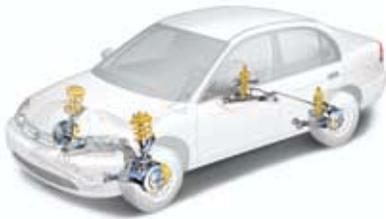
Civic Coupe's front MacPherson strut and rear double wishbone suspensions with a high-mounted steering system are designed to absorb bumps without compromising stability for smooth, controlled ride qualities.
