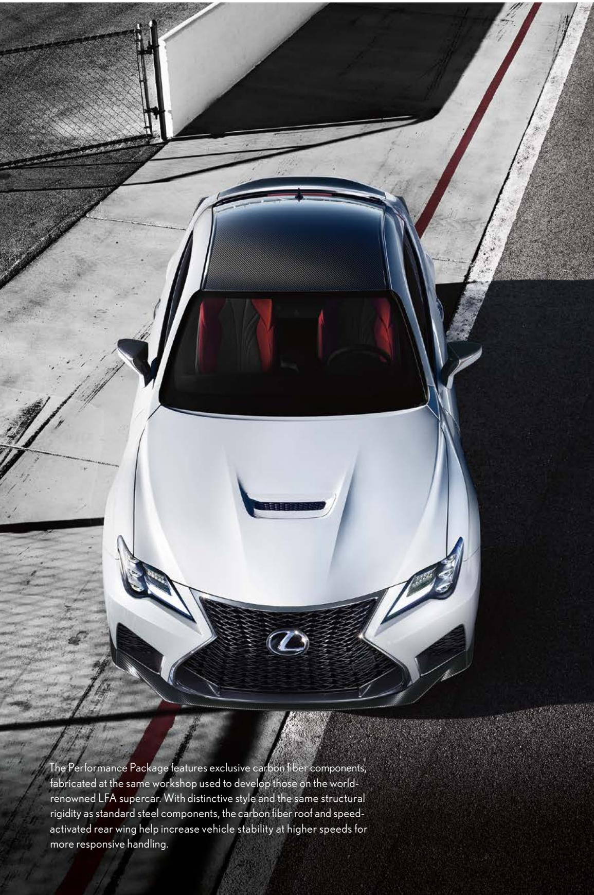
The Performance Package features exclusive carbon fiber components, fabricated at the same workshop used to develop those on the world-renowned LFA supercar. With distinctive style and the same structural rigidity as standard steel components, the carbon fiber roof and speed-activated rear wing help increase vehicle stability at higher speeds for more responsive handling.
