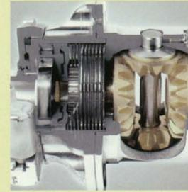
Steep, rough or slippery roads? No sweat. Switch into 4WD Low to lock the Quadra-Drive II transfer case clutch pack. Engine torque is multiplied 2.72 times. Available.
