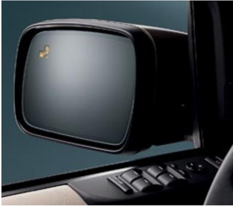
Side-mounted radar gives the available Blind Spot Monitoring system the ability to warn of vehicles that the driver may not see. A bright amber warning icon is illuminated in the appropriate door mirror when a hazard is detected.
