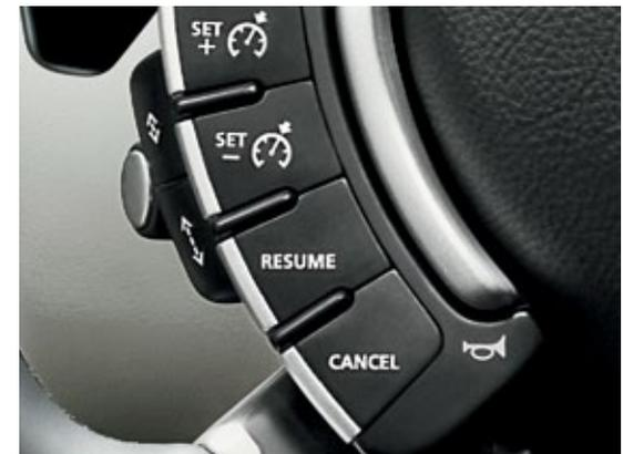
Available Adaptive Cruise Control has four driver-selectable settings, designed to suit individual driving styles and traffic/road conditions.
