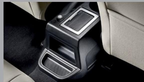
**CENTER CONSOLE STORAGE.** The rear of the center console features an additional storage box for small items, a 3.5mm auxiliary socket for MP3 players and a power socket, which can be used to recharge PCs and low-wattage electrical equipment.
