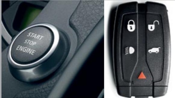
**START/STOP BUTTON AND REMOTE CONTROL.** In order to start the car the remote has to be docked into the fascia and the correct procedure followed using the Start/Stop button. The remote control includes the following functions: locking and unlocking of the doors and tailgate, a 30 second courtesy headlamp delay and activation of panic alarm.
