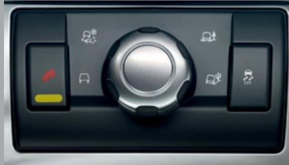
**TERRAIN RESPONSE®.** Land Rover's patented Terrain Response® system adds to the Land Rover LR2 vehicles breadth of capability. Any of the four settings – general driving, grass/gravel/snow, mud and ruts, or sand – can be easily selected by simply turning the rotary control. In addition all vehicles with Terrain Response® are also fitted with Land Rover's Hill Descent Control (HDC®) and Gradient Release Control systems.
