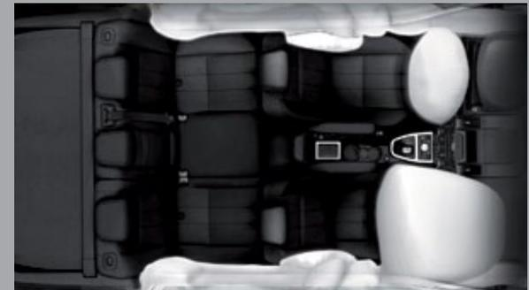
**SAFETY\*\*.** High-strength steel is used to construct a strong monocoque body and inner safety cell protected by front and rear energy absorbent crumple zones. Seven airbags are fitted as standard on all vehicles.
