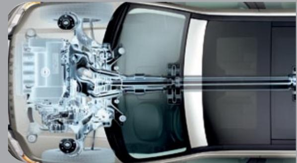
**PERFORMANCE WITH REFINEMENT.** A compact, advanced 3.2 liter in-line straight-six engine with Cam Profile Switching and Variable Valve Timing delivering more power, a better spread of torque and greater efficiency.
