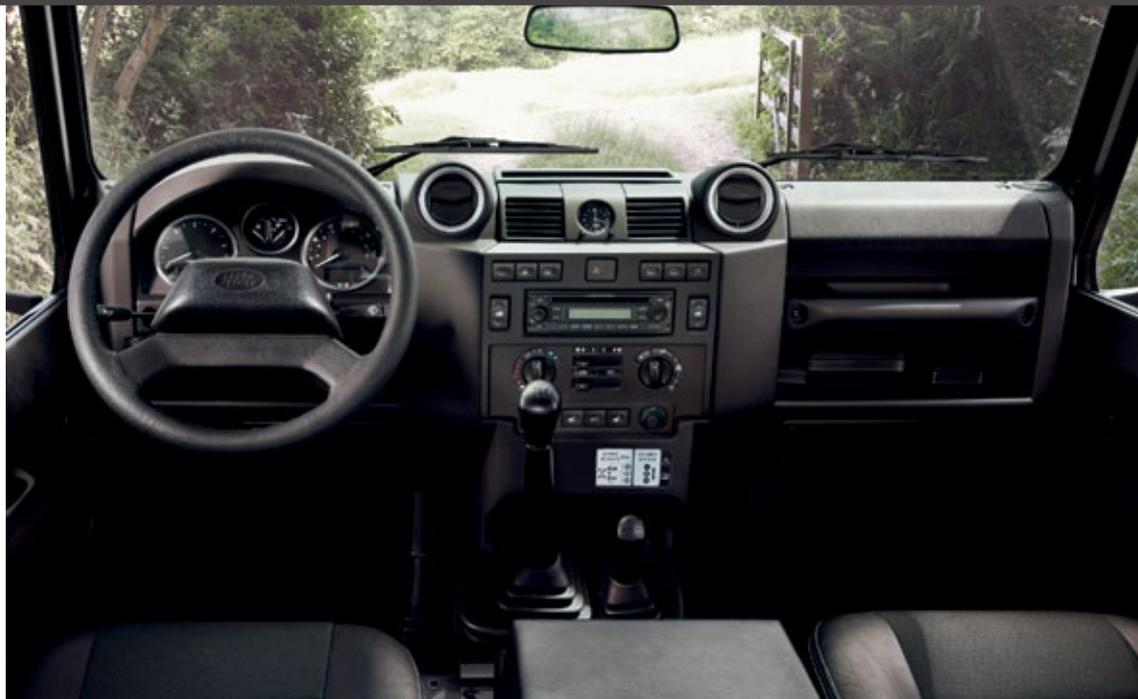
Form follows function in the Defender interior. Tough working vehicles demand robust materials such as the scuff-resistant fascia and durable seat coverings. The fascia is a one-piece moulding for improved refinement, its distinctive lines providing Land Rover's traditional commanding view of the ground ahead.
