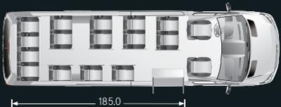
Select from multiple interior seating configurations for the Sprinter MiniBus.
