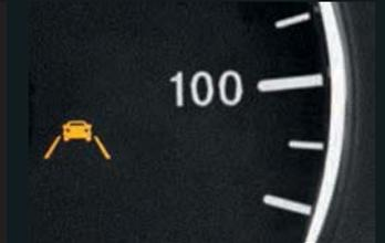
Lane Keeping Assist<sup>®11</sup> provides the driver with audible and visible warnings if the vehicle leaves its lane unintentionally. A camera in the windshield monitors the road ahead and helps detect when you may veer away from lane markings.
