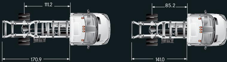
Choose between two wheelbases (144 inches and 170 inches—both with GVWRs of 11,030 pounds), and build the Sprinter Cab Chassis/Cutaway that works best for you.
