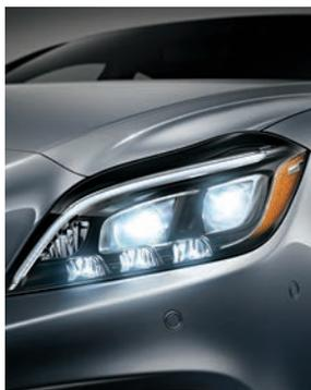
**Leading with LEDs.** The CLS employs brilliantly efficient LED technology for virtually all of its exterior lighting, from its full-LED headlamps to its taillamps. The available new ACTIVE MULTIBEAM LED<sup>®</sup> headlamps maximize illumination without causing glare for other drivers. They shift their beams into curves, and precisely adapt their high beams based on continuous camera scanning. They can also help brighten low-speed turns into dark driveways, alleys or garages.
