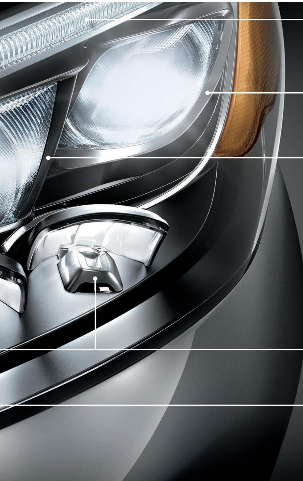
**Multicolor/multifunction fiber-optic LED.** The distinctive, continuous arch over the headlamp serves as the bright white Daytime Running Lamp, the more softly glowing parking lamp, or the flashing amber turn signal. Day or night, its shape seamlessly flows into the signature character line in the side profile of the CLS.
