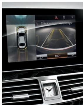
**A better view of what's around you.** An available rearview camera shows a live view of what's just behind your vehicle on the central in-dash screen. Active steering guidelines help you back smoothly into a parking space. The optional Surround View System uses four cameras to create a single live "birds-eye" view of your immediate surroundings. It helps you maneuver more easily in tight spaces, whether you're moving forward or backing up.<sup>10</sup>
