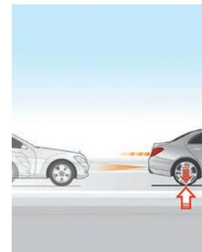
**Action when danger is behind you.** Part of the Driver Assistance Package, PRE-SAFE<sup>®</sup> PLUS uses radar to sense a possible rear-end collision before it occurs. If it senses you're about to be hit from behind, it can tighten the front seat belts. If you're already stopped, it can firmly apply the brakes to help minimize whiplash injuries. It can also hold the brakes after impact, to help prevent a secondary collision even if the driver's foot slips off the brake.<sup>7</sup>
