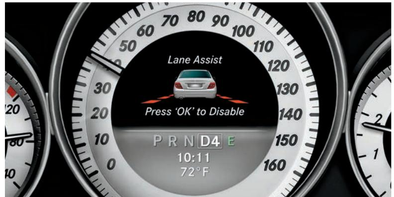
**Multilane multitasker.** Optional Active Lane Keeping Assist uses a camera to monitor the car's position in relation to visible lane markings. If you start to drift out of your lane without using a turn signal, it can alert you by vibrating the steering wheel. If you disregard the system's alerts, its advanced active technology can also gently apply the brakes to individual wheels, to help draw the vehicle back into its original lane.<sup>8</sup>
