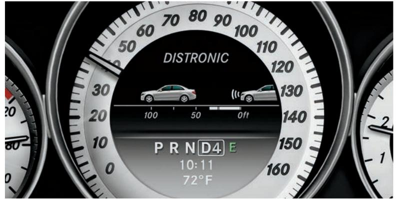
**Cruise control that stops and goes.** Available DISTRONIC PLUS<sup>®</sup> uses radar to adapt your set cruising speed in response to the flow of traffic ahead. It can slow the vehicle automatically—or brake to a full stop—then resume with a tap.<sup>5</sup> Even if you're not using cruise control, PRE-SAFE<sup>®</sup> Brake can alert you to stopped traffic, and automatically apply up to 100% braking force to help prevent or reduce the severity of an impact.<sup>7</sup>
