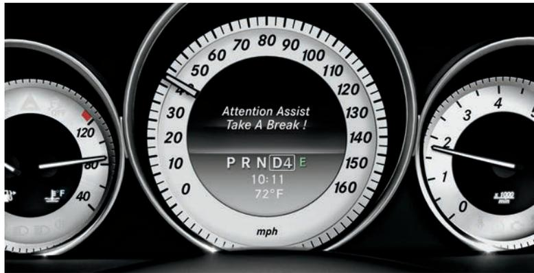
**A watchful eye when's it time for a rest.** ATTENTION ASSIST<sup>®</sup> is a Mercedes-Benz innovation that can alert you if it detects signs of drowsiness on long drives. It measures more than 70 variables, starting in the first minutes of a drive, to establish a pattern. By continually monitoring a variety of driving behaviors along your trip, it can offer a warning tone and encourage taking a rest if it senses you're getting drowsy.<sup>8</sup>
