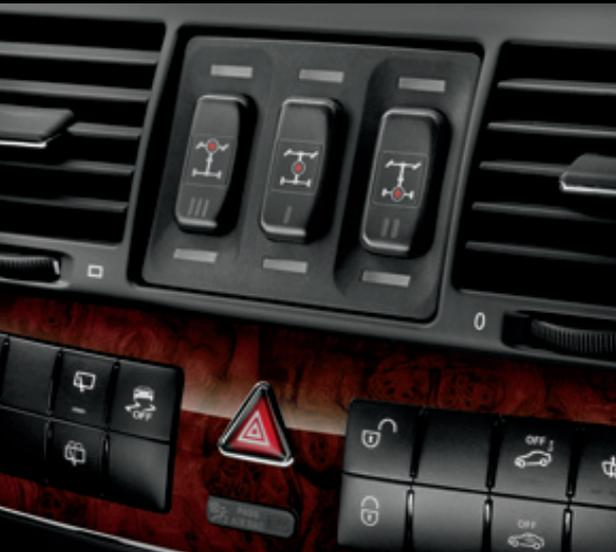
**Off-road prowess.** Each of the three differentials can be locked in sequence—center, rear, then front—via a set of buttons on the dash. With more than eight inches of both ground clearance and suspension travel, along with steep angles of approach and departure, the G-Class can venture where most other SUVs can only dream. It can even climb or descend an 80% incline, and handle a 54% lateral slope.<sup>4</sup>
