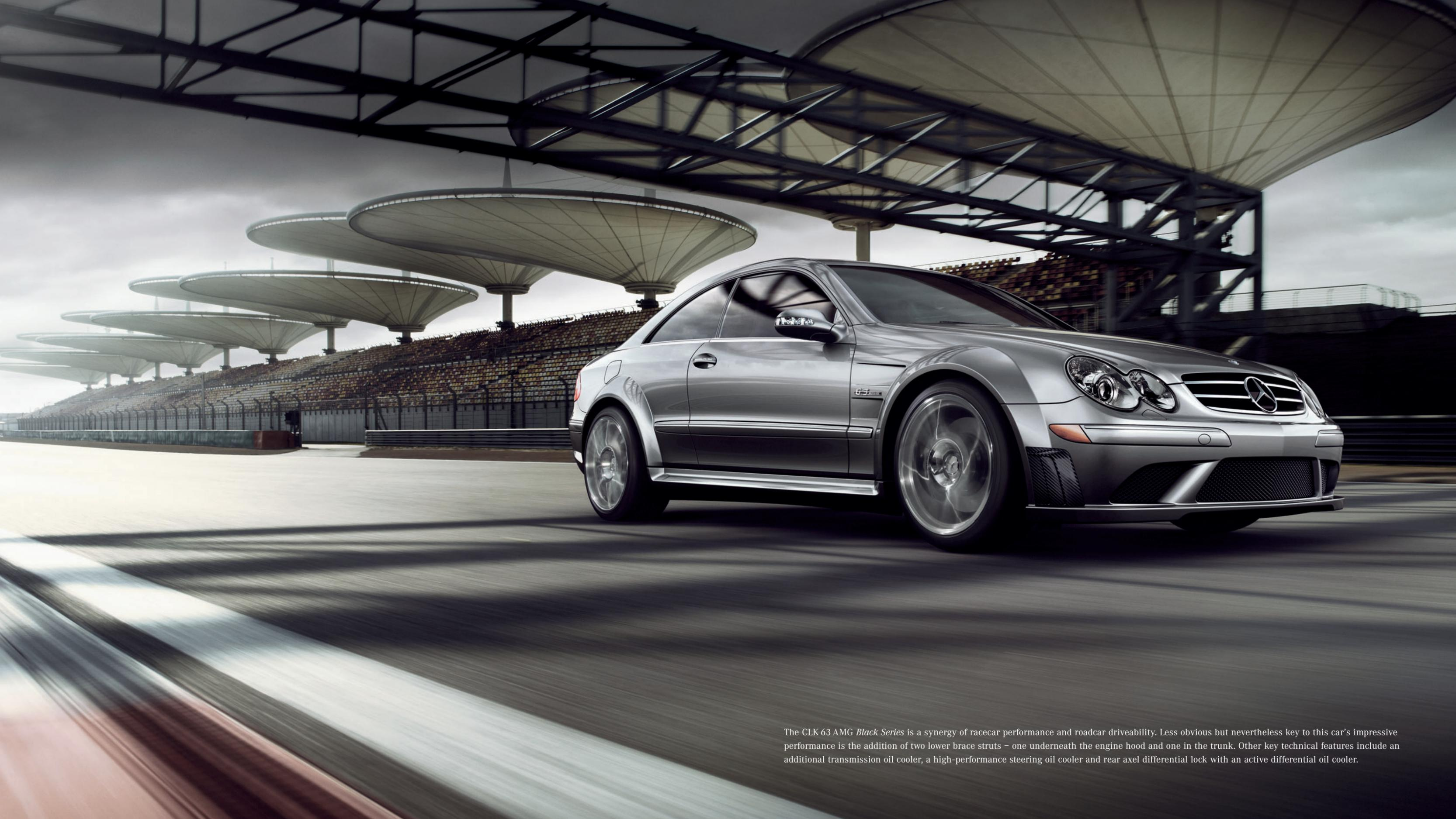
The CLK 63 AMG *Black Series* is a synergy of racecar performance and roadcar driveability. Less obvious but nevertheless key to this car's impressive performance is the addition of two lower brace struts – one underneath the engine hood and one in the trunk. Other key technical features include an additional transmission oil cooler, a high-performance steering oil cooler and rear axel differential lock with an active differential oil cooler.
