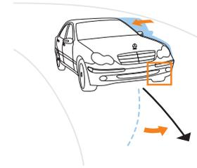
B. ESP brakes the inside rear wheel to address understeer.
