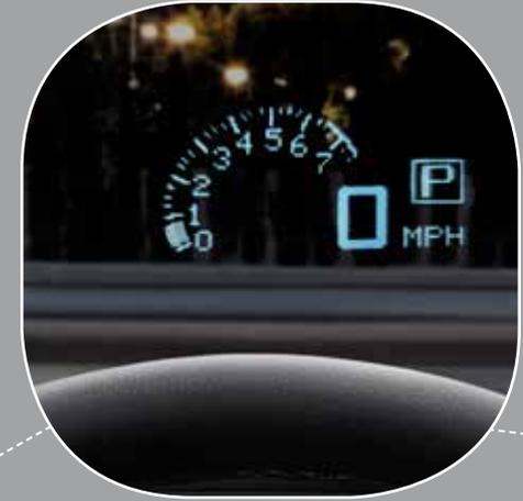
**HEAD-UP DISPLAY** This standard system projects important driving information at eye level on your windshield, such as speedometer, audio information, outside air temperature and more.
