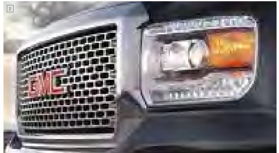
**2 SIGNATURE LIGHTING** In a GMC pickup first, Sierra introduces a new projector-beam headlamp fully integrated into the grille surround. The headlamps create a bold, distinctive appearance, further enhanced with available LED signature lighting (standard on SLT and Denali).
