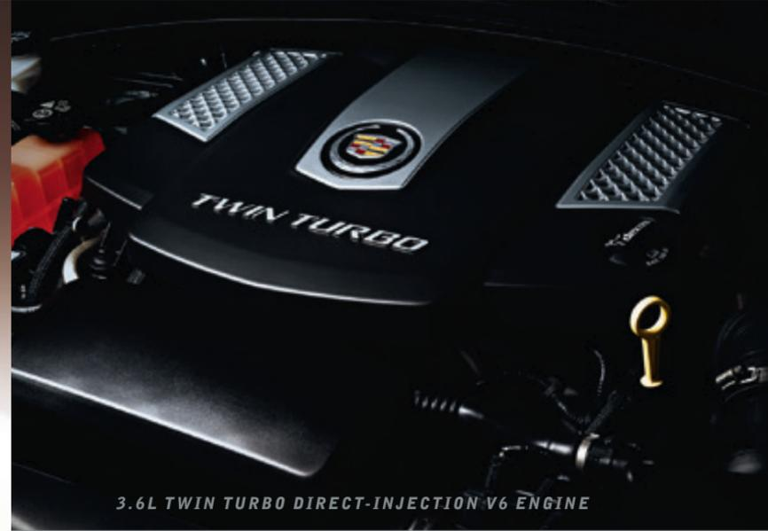
3.6L TWIN TURBO DIRECT-INJECTION V6 ENGINE
