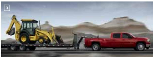
**UP TO 18,000 LBS CONVENTIONAL TRAILERING** Available 2.5" trailer-hitch receiver enables up to 18,000 lbs maximum conventional towing capacity (2" adapter included).<sup>2</sup>
