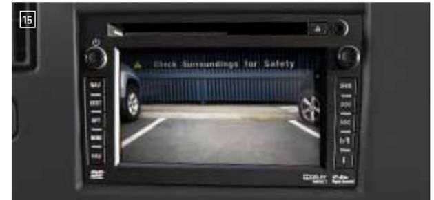
**15 REAR-VISION CAMERA SYSTEM** This available system places a monitor in your rearview mirror (or navigation screen, if equipped) to display a view of the area behind the vehicle, making it easier to back up to a trailer or negotiate a tight space.
