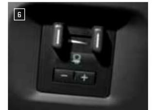
**6 INTEGRATED TRAILER-BRAKE CONTROLLER** Provides immediate and measured brake-force signaling to electric-controlled trailer brake systems. Available on Sierra WT and SLE models.
