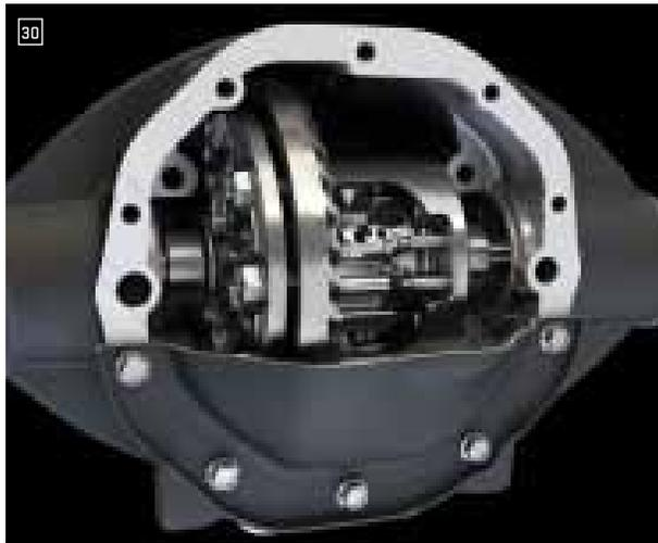
**30 EATON® HEAVY-DUTY AUTOMATIC LOCKING REAR DIFFERENTIAL** When the Eaton locker senses the difference in rotational speed between left and right wheels of approximately 100 rpm, it locks the differential to turn both wheels in unison for added traction. Standard on Yukon and available on Sierra and Savana, no other competitors in their class offer this automatic locking rear differential for on- or off-road use.
