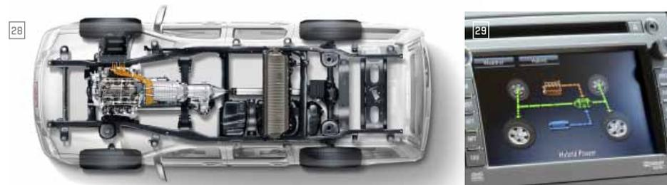
**28 HYBRID POWERTRAIN** The Two-Mode Hybrid System saves fuel with an all-electric launch, low-speed electric-only propulsion and electric assist during demanding driving. It is comprised of a Vortec 6.0L VVT V-8 engine, two 60-kilowatt electric motors housed within the transmission that also act as generators, a 300-volt battery that powers the system and an innovative regenerative braking system that results in an EPA-estimated 20 mpg city/23 mpg highway for both Sierra and Yukon.
