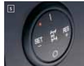
**5 AVAILABLE POWER TAKEOFF (PTO)** Sierra 3500HD Chassis Cab models equipped with the available Allison<sup>®</sup> automatic transmission have a dash-mounted PTO control to accommodate an aftermarket PTO to drive equipment such as a hydraulic dump body, hydraulic pumps or generators.
