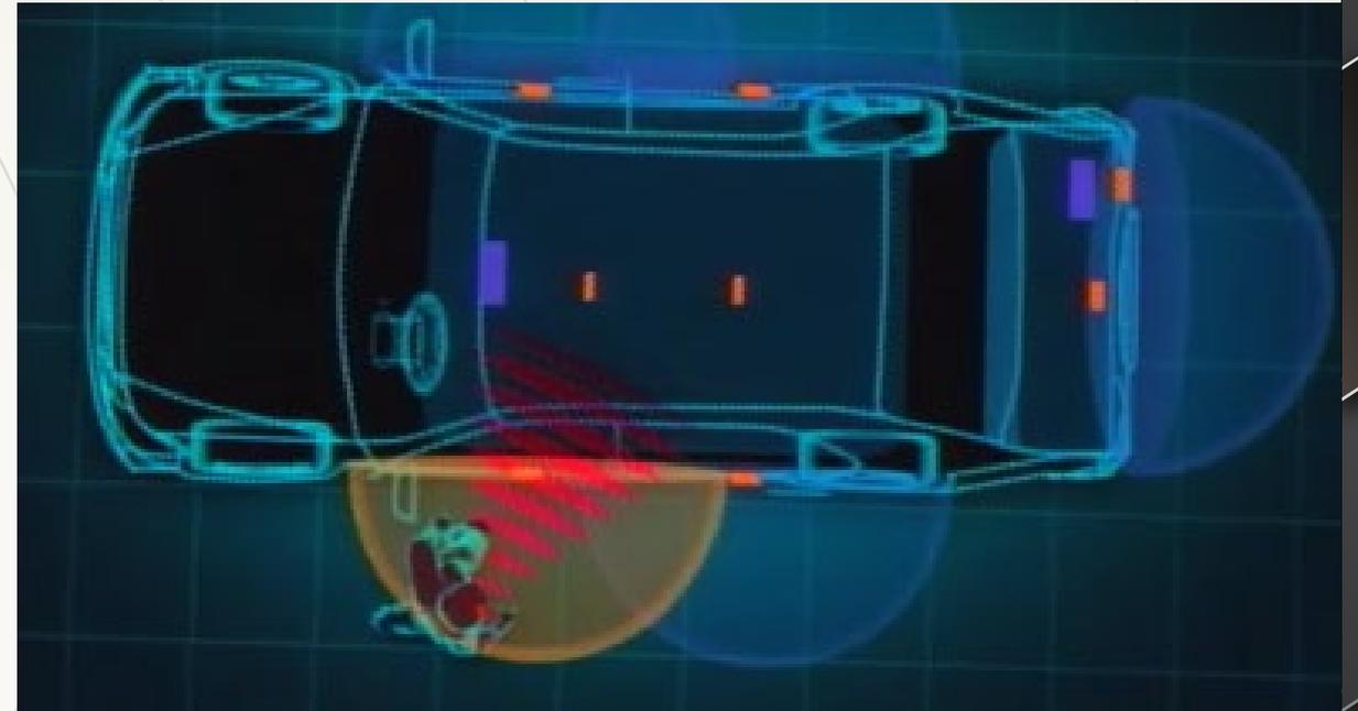
As you approach your IS, SmartAccess<sup>9,10</sup> automatically transmits a secure signal directly from your key fob activating the vehicle's lighting sequence and illuminating points of entry—the first being the exterior puddle lights. When your hand touches the door handle,
