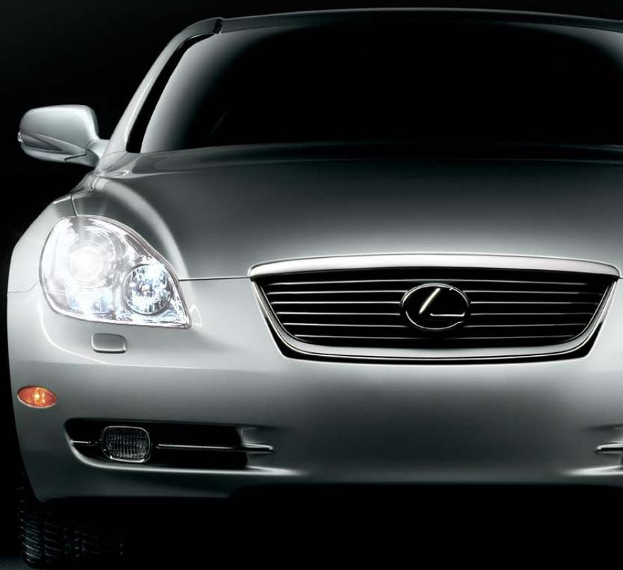
While the jeweled-cluster headlamps on the SC are attractive in their own right, they actually serve a purpose. To help illuminate more of the road through turns, the Adaptive Front Lighting System (AFS) can pivot the left headlamp up to 15 degrees and the right headlamp up to 5 degrees into a curve. And to help reduce glare to oncoming traffic, dynamic auto-leveling High-Intensity Discharge (HID) headlamps automatically sense and adjust to changes in load and road conditions.
