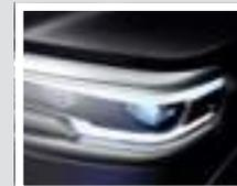
**AVAILABLE SMARTBEAM HEADLAMPS†** This advanced system provides the maximum amount of light possible, automatically switching headlamps from high- to low-beam when oncoming headlamps or forward light is sensed, or when taillamps are detected in front of the vehicle.
