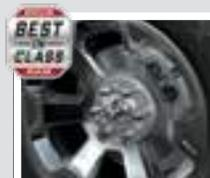
**THE LARGEST STANDARD BRAKES IN THE SEGMENT†** Confident stopping power comes from a new brake system. The new brakes have the largest standard rotors in the segment†, measuring nearly 15 inches in diameter fore and aft, sharply reducing 60-0 mph stopping distances and improving performance.
