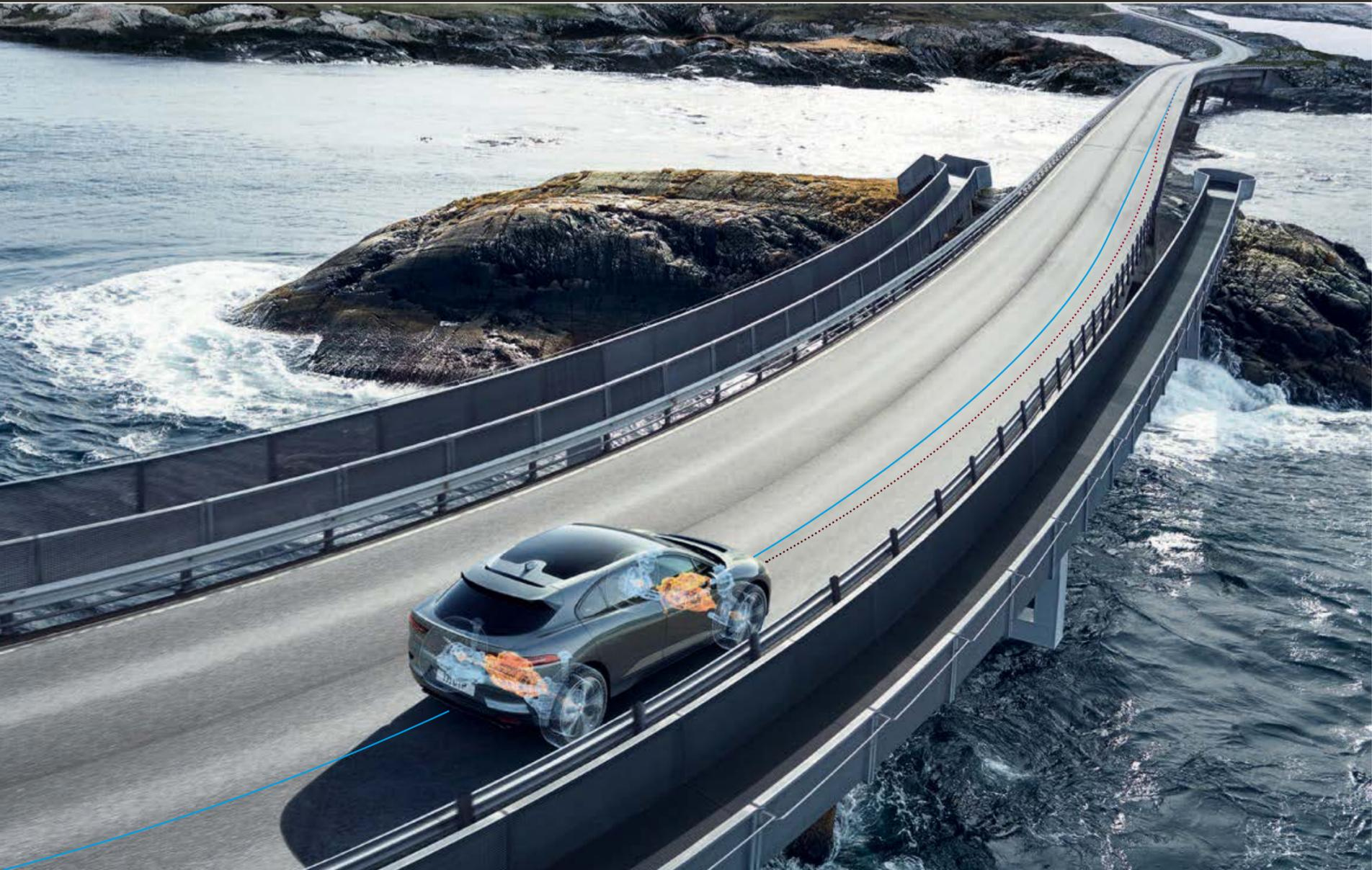
Torque Vectoring by Braking applies brake pressure to slow the inside front or inside rear wheels independently helping to prevent understeer and stay on the true line of travel.
