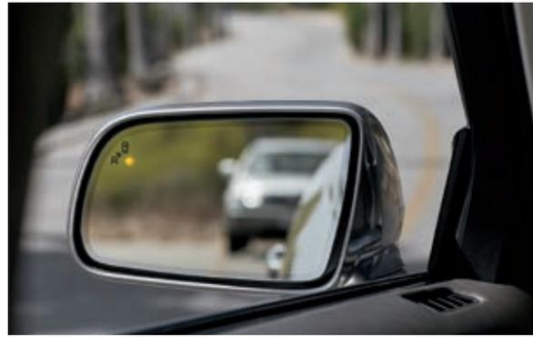
**BLIS® (BLIND SPOT INFORMATION SYSTEM) WITH CROSS-TRAFFIC ALERT<sup>1,2</sup>** – Some vehicles may be out of your line of sight, but they can be detected by this technology. It warns you if it detects a vehicle in your blind spots while driving forward, or approaching from the sides while in Reverse.
