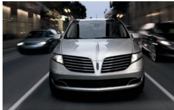
**ADAPTIVE HID HEADLAMPS** – Paired with convenient auto high beams, these sophisticated headlamps feature bright-white light that provides better visibility than conventional halogen lamps. Their beams also move in the same direction as the steering wheel for more visibility when driving around curves.
