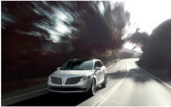
**LANE-KEEPING SYSTEM<sup>1,2</sup>** – If you start to drift out of your lane, this technology can help. Using a forward-facing camera to detect road lane markings, the system can apply steering wheel torque and even alert you with a steering wheel vibration to help direct you to return to your lane.<sup>3</sup> If it detects that you've crossed the line repeatedly, it can prompt the Driver Alert System<sup>1,2</sup> to chime and display a coffee cup image to remind you that it's break time.
