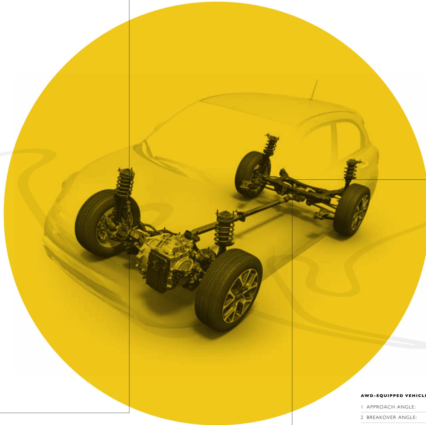
FIAT® 500X is the first in the 500 family to offer the confidence of All-Wheel Drive (AWD), and this new generation drive system brings new functionality and improvements over conventional AWD systems. It features a disconnecting rear axle that helps to improve fuel efficiency by automatically selecting Front-Wheel Drive (FWD) or AWD when necessary. It completely removes power to the rear axle when FWD performance is adequate during regular conditions.
