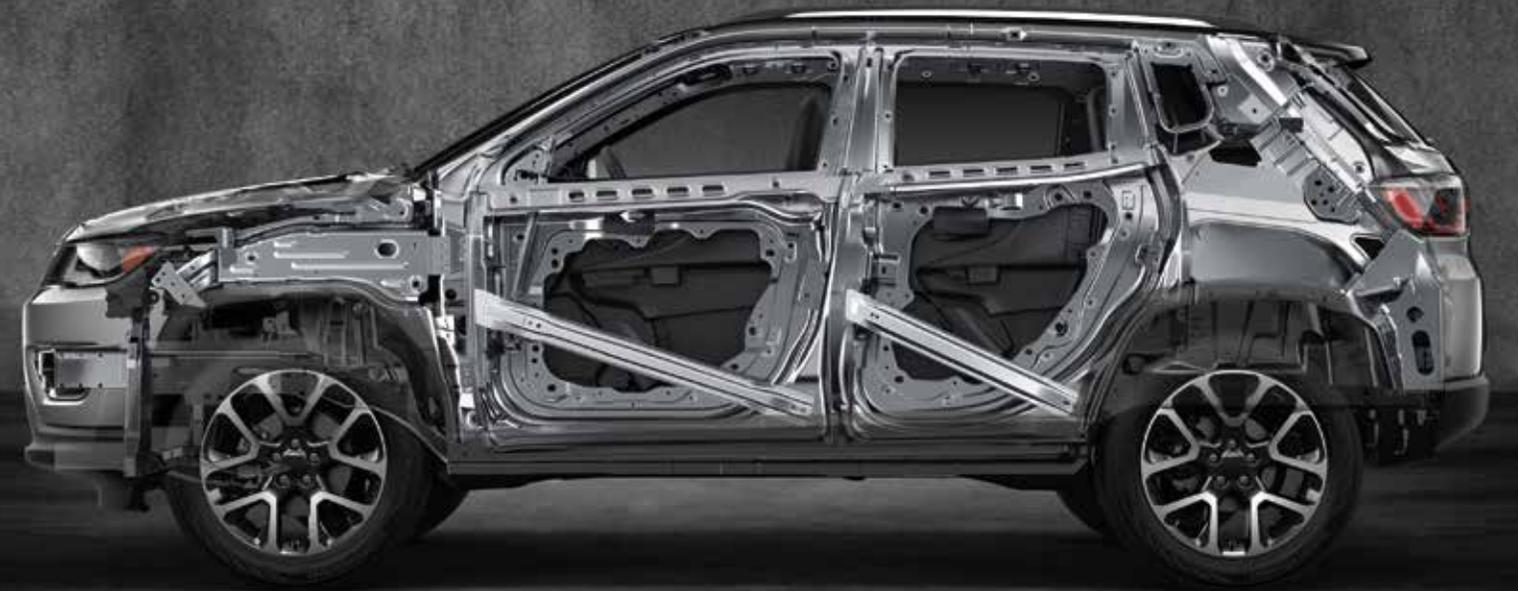
**CHASSIS STRENGTH** COMPASS DELIVERS EXCEPTIONAL PEACE OF MIND WITH A HERO'S HEART — A STRONG UNIBODY STRUCTURE IS ENGINEERED WITH APPROXIMATELY 70% HOT-STAMPED STEEL. STANDARD.
