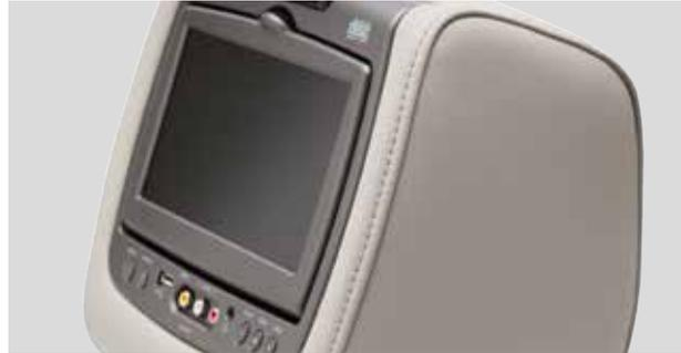
**REAR-SEAT ENTERTAINMENT SYSTEM** The system has dual LCD monitors and DVD players mounted on the rear of the front-seat head restraints. Wireless headphones and a remote control allow rear passengers to enjoy the audio. Includes USB and RCA inputs.<sup>1</sup>
