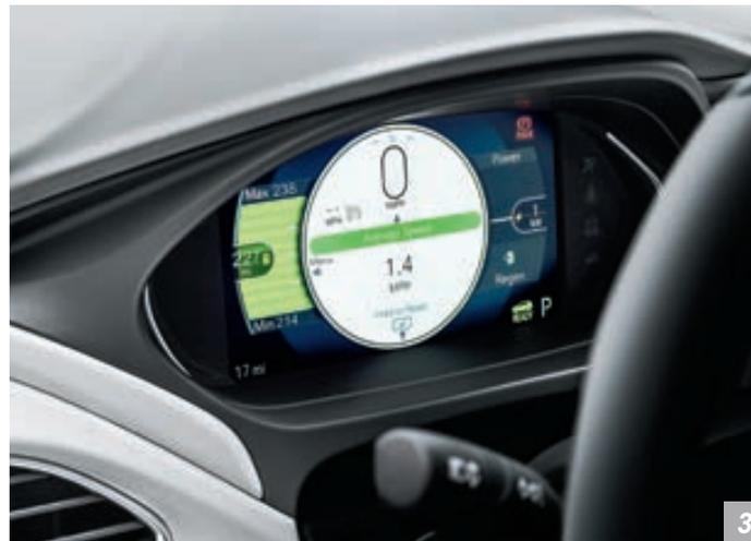
**3. RANGE ANALYSIS.** A Confidence Gauge in the configurable Driver Information Center provides best-case and worst-case scenarios based on recent driving conditions. It analyzes how you trend on efficiency based on real-life driving information.
