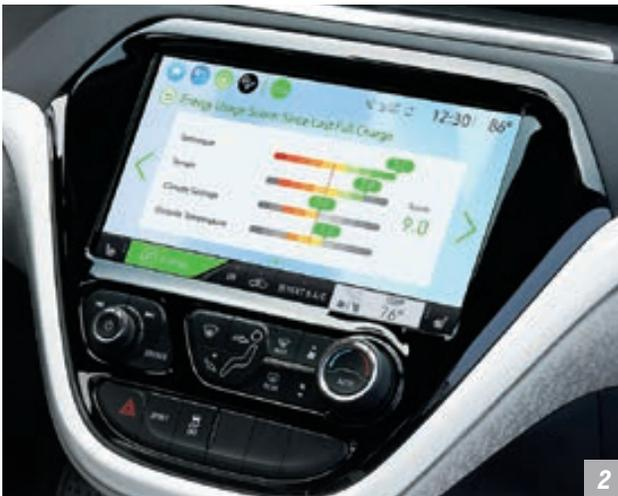
**2. ENERGY USAGE SCREEN.** This screen breaks down the percentage of energy used for driving, climate control and battery conditioning. See how much energy you're using when adjusting heat or air conditioning settings to control your comfort level.
