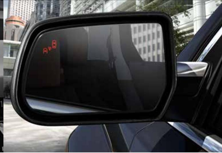
**SIDE BLIND ZONE AND REAR CROSS TRAFFIC ALERTS** Available radar-equipped sensors monitor side blind spots (shown above), alerting you to help reduce the risk of collisions. While in reverse, the available Rear Cross Traffic Alert monitors your surroundings to provide visual and audible alerts to traffic approaching from outside your field of vision.
